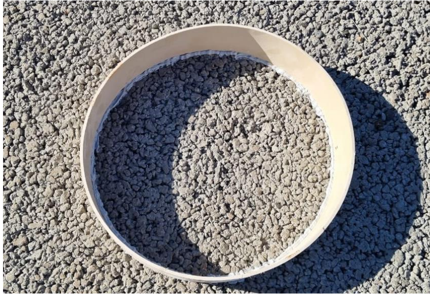
Figure 6 - PVC pipe ring used in the permeability test. Source: Author himself.
